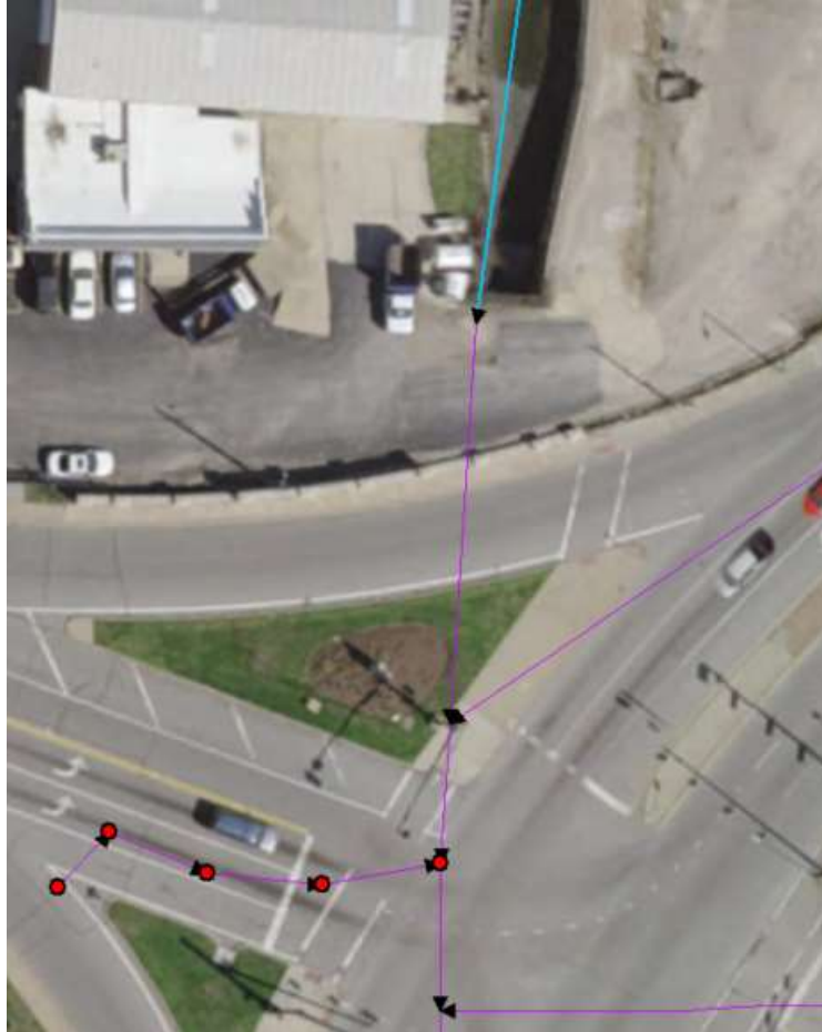
Figure 49 - Example of missing Hydrojunction at end of Stream
