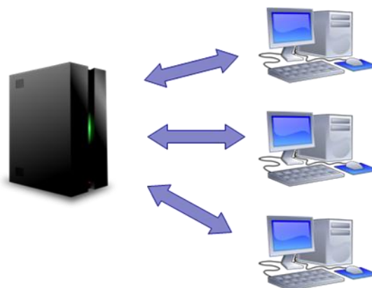
Figure 2. Conventional approach: many workstations and one server
