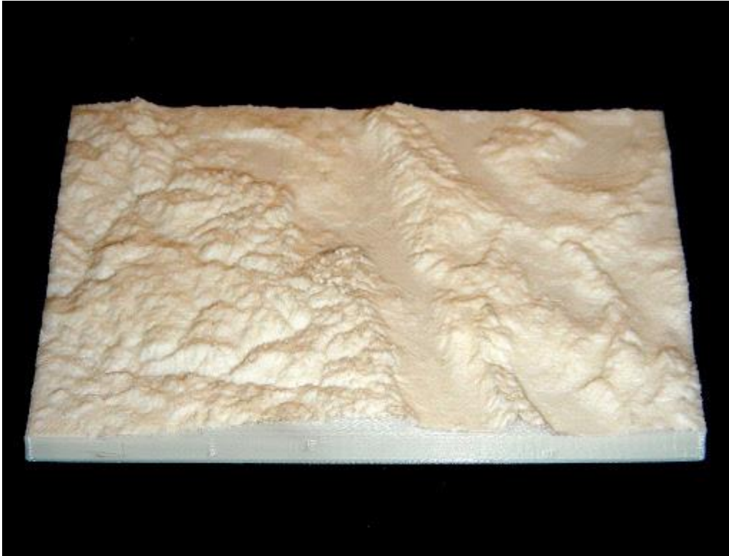
L. The final product - a 3D printed topographic map
