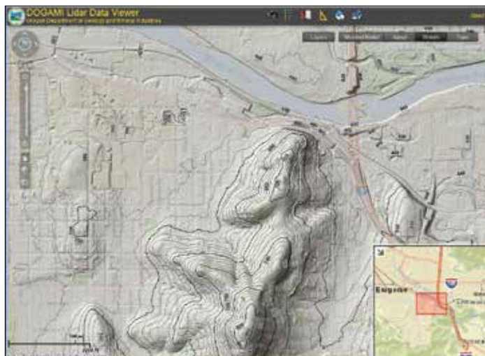
↑ Lidar data is used to create bare-earth DEM representations that exclude man-made structures and vegetation.
