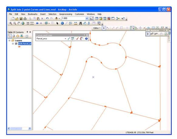
Example 2: the single line feature is split into 7 features; five circular arcs, and two 2-point lines.
