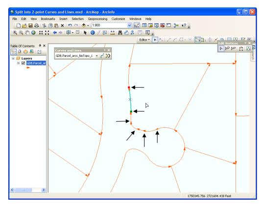
Example 3: the single line feature is split into multiple 2-point lines.
