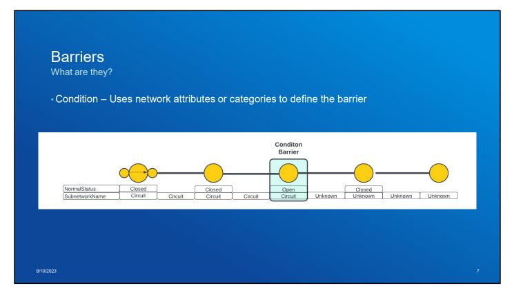
Condition Barriers are where we use attribute values to determine if something is a barriers, like a switchable device being open. When the trace encounters a feature with this attribute set to Open, it will stop.
