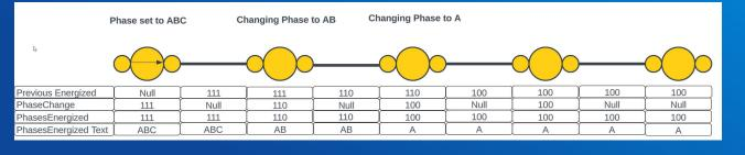
PhasesEnergized from previous object is and'd with PhaseChange of the current object to calculate the new Phases Energized value
