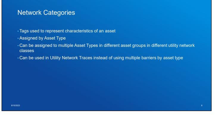
We have used network categories extensively in the EUNF model. Categories are assigned at the asset type level and have a performance advantage in tracing because of that.
