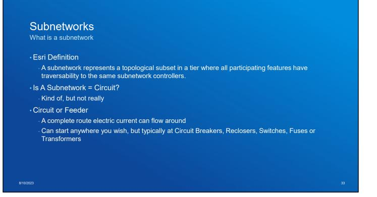
Is a subnetwork a Circuit, well kind of, but not necessarily. We will go deeper in to Subnetworks
