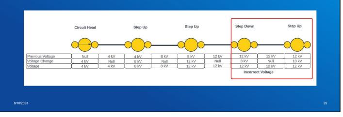
As you saw from these two examples of voltage propagation, you can get the incorrect voltage propagated when you have a mix of Step Up and Step Down Transformers
