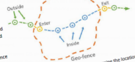
Figure 1: Use of a spatial filter to determine the location of a moving asset in relation to a geo-fenced area
