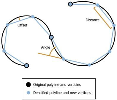
The curve is densified into linear segments by either the Offset, Distance, or Angle.
