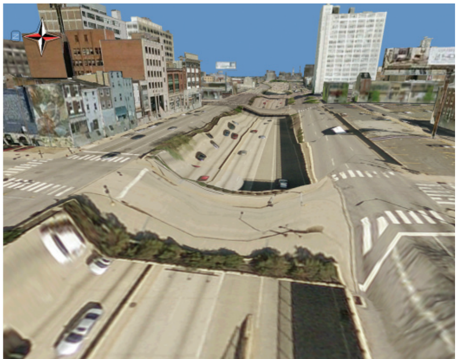
Figure 1: This exercise shows how to correct this sampling error, commonly seen in high-resolution DEMs in urban environments.
