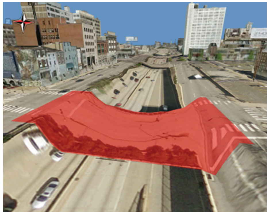
Figure 3: By default, the polygon will drape over the globe surface like a blanket.
